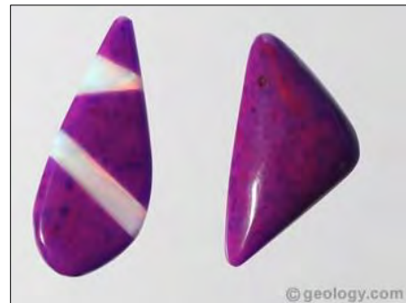
The purple material in these cabochons is made of powdered sugilite that has been pressed into a mold and bound together by resin. The cabochon on the left is an assembled stone made by artistically combining imitation sugilite and imitation opal. The cab on the left measures 20 x 50 millimeters, and the cab on the right measures 23 x 45 millimeters.
