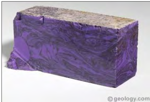
A block of imitation sugilite made from a resin composite. This specimen measures approximately 9.8 x 4.8 x 3.5 centimeters.
