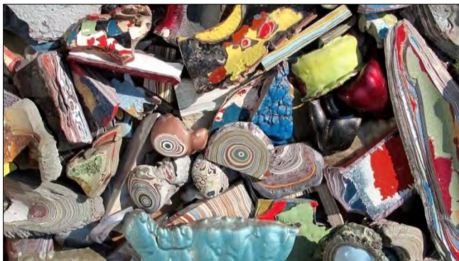
Fordite rough shows layers of automotive paint.
